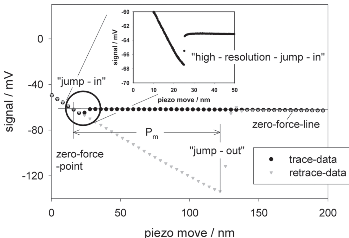
FIGURE 1 Measured force-distance-curve with low and high resolution. The adhesion force of a particle can be calculated by multiplying the distance, P_m , by the spring constant of the cantilever.
